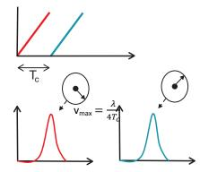
Figure 6. Two-chirp velocity measurement.
