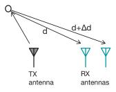
Figure 11. Two antennas are required to estimate AoA.
