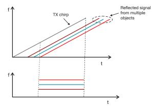
Figure 5. Multiple IF tones for multiple-object detection.
