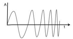
Figure 1. Chirp signal, with amplitude as a function of time.
