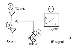
Figure 3. FMCW radar block diagram.
