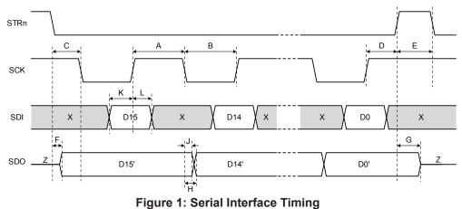
X = do not exceed Watchdog Config timeout; Z = high-impedance (tri-state)
