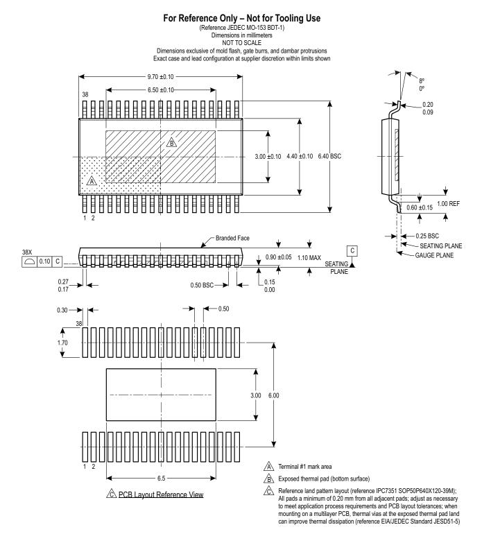
Figure 10: Package LV, 38-Pin eTSSOP
