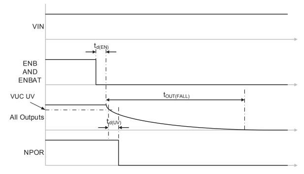
All outputs start to decay  $t_{d(EN)}$  seconds after ENB and ENBAT are low.
