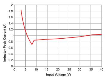
Figure 8: Typical Peak Inductor Current versus Input Voltage for 0.8 A Output Current and 10  $\mu H$  Inductor
