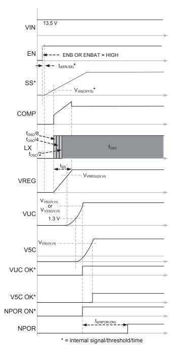
Figure 2: Startup Timing Diagram
