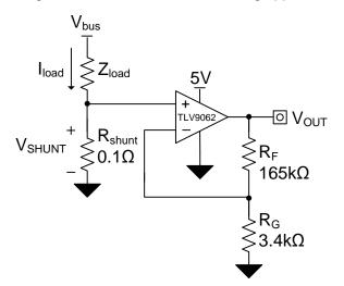
Figure 37. TLV906x in a Low-Side, Current-Sensing Application
