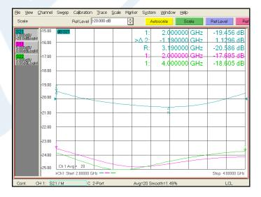
Click the following link (or enter part number in "SEARCH" on website) to obtain additional part information including price, inventory and certifications: 0 to 60 dB Voltage Variable Attenuator, PIN Diode, 2 GHz To 4 GHz, SMA PE70A2000
