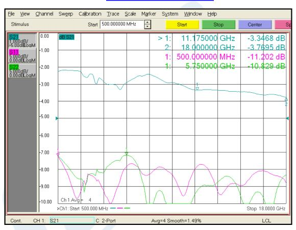
Click the following link (or enter part number in "SEARCH" on website) to obtain additional part information including price, inventory and certifications: 0 to 60 dB Voltage Variable Attenuator, PIN Diode, 500 MHz To 18 GHz, Rated To 0.1 Watts, SMA PE70A2900
