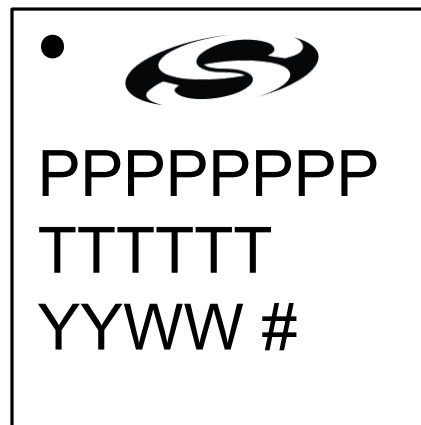
Figure 6.3. QFN28 Package Marking
