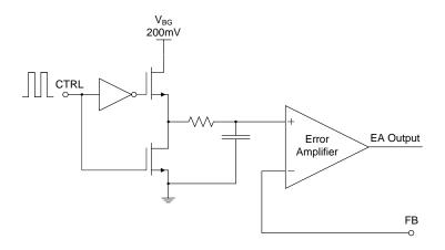
Figure 2. Block Diagram of Programmable FB Voltage in PWM Dimming Mode
